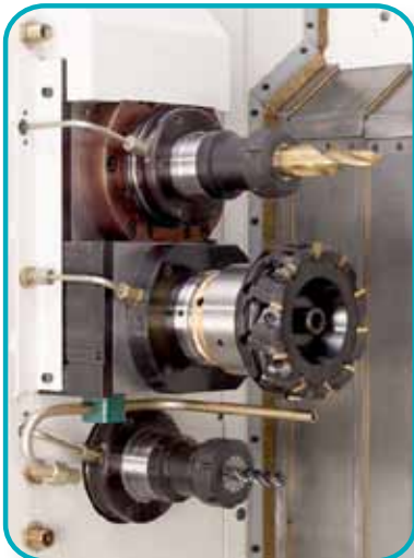
Machining unit with three spindles.
