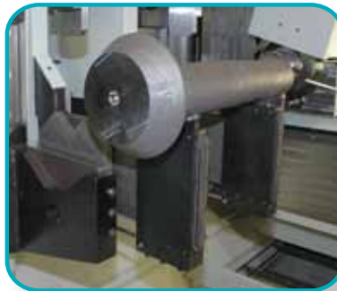
Part prelocators, nc controlled automatically in height adjustable.
