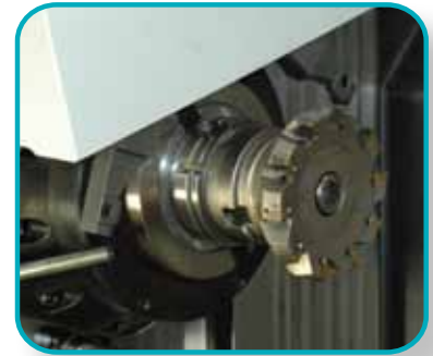
Automatic tool changer with double gripper.
