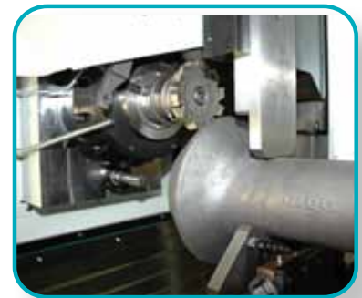
Central working clamping devices, for 3-point or 4-point clamping.
