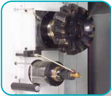
Machining unit with two spindles.
