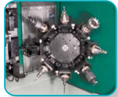
Machining units with 4-, 6-, 8-fold turrets for shortest chip to chip time.
