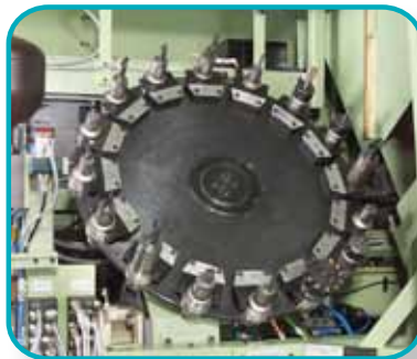
Tool magazines, executed as 8- or 16-fold disc magazines.
