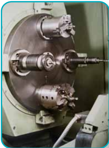
Rigid machining unit with 4-fold disc magazine.
