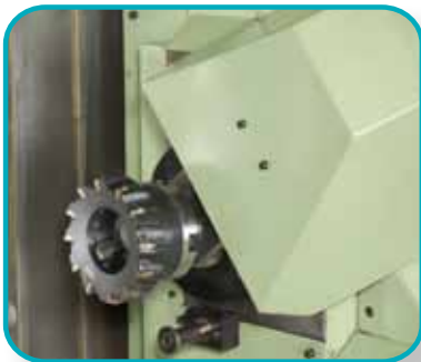
Automatic tool changer with double gripper.
