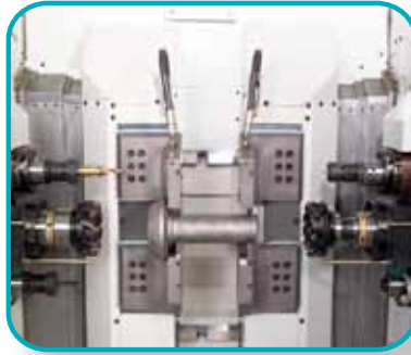
Machining units with 1,2 or 3 spindles
