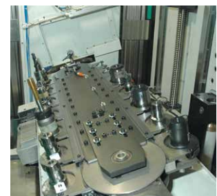
Tool magazines, executed as 8-, 16-, 24- or 32-fold chain magazine
