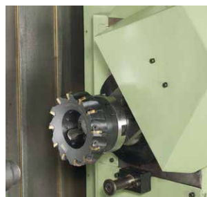
Automatic tool changer with double gripper
