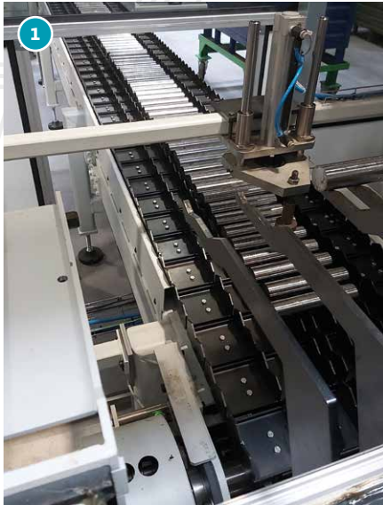
1) FEED CONVEYOR BELT with lifting and shaft inspection for diameter and length
