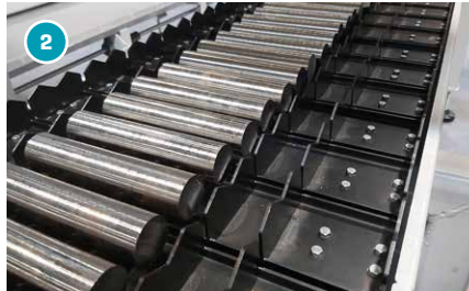
2) CONVEYOR BELT with cassette conveyor chain for variable diameters and lengths
