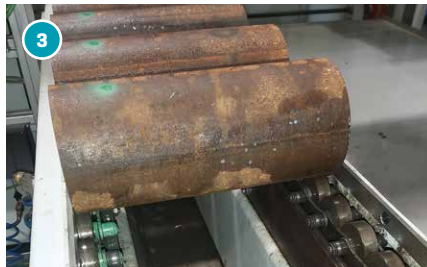
3) DISCHARGE CONVEYOR BELT Roller belt with width adjustment for variable diameters and lengths
