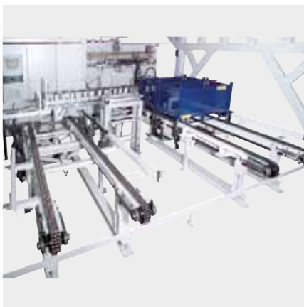
Representation of the loading and unloading conveyor section
